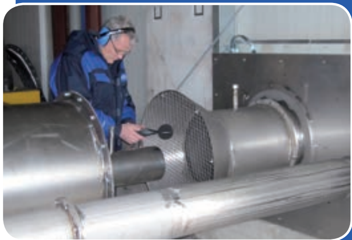
Measuring sound levels from the Nießing test bench
