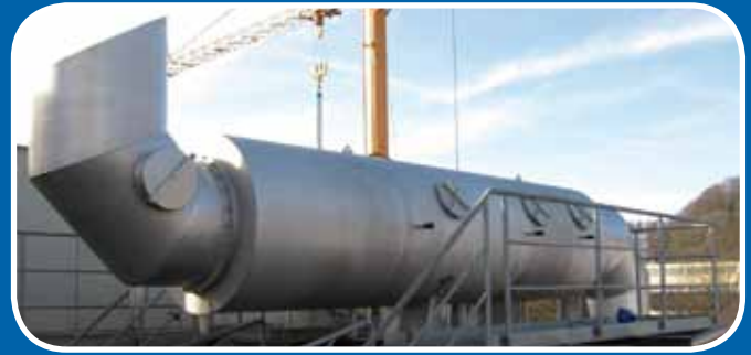
Volume resonator with cleaning facility
